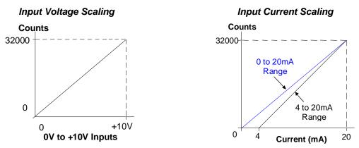
If the current source is reversed into the input, or is less than the low end of the current range, the module inputs a data word corresponding to the low end of the current range (0000H in %AI). If an input is out of range (greater than 20 mA), the A/D converter adjusts it to full scale (corresponding to 7FFFH in %AI).
