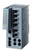
SCALANCE XC206-2 managed Layer 2 IE switch; IEC 62443-4-2 certified; 6x 100 Mbps RJ45 ports; 2x 100 Mbps ST/BFOC ports; 1x console port; diagnostics LED; redundant power supply; temp. range -40 °C to +70 °C; mounting: DIN rail/S7 mounting rail/wall redundancy functions; Office features (RSTP, VLAN,...); PROFINET IO device; Ethernet/IP-compliant C-plug slot;
