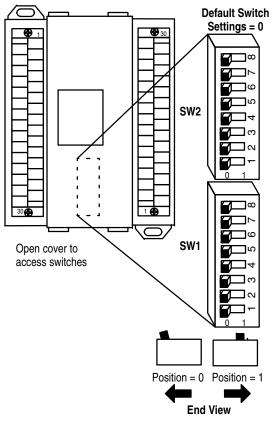
**ATTENTION:** Cycle power to the module after setting the switches.
