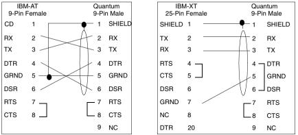
Modbus Ports Pinout Connections for Portable Computers
